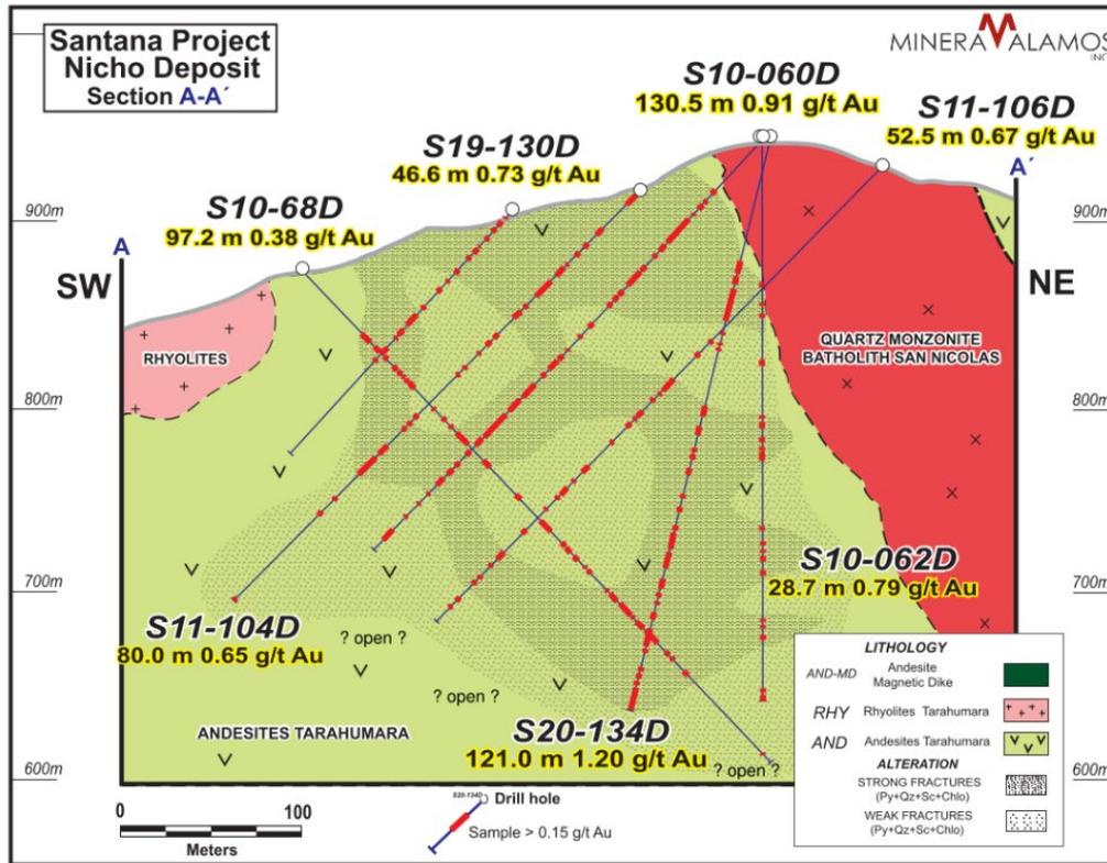
Note: Grade/width of composite intervals is a total of all mineralized intervals that have gold grades equal to or in excess of “typical” open-pit mining heap leach cut-off grades of 0.15 g/t gold.
