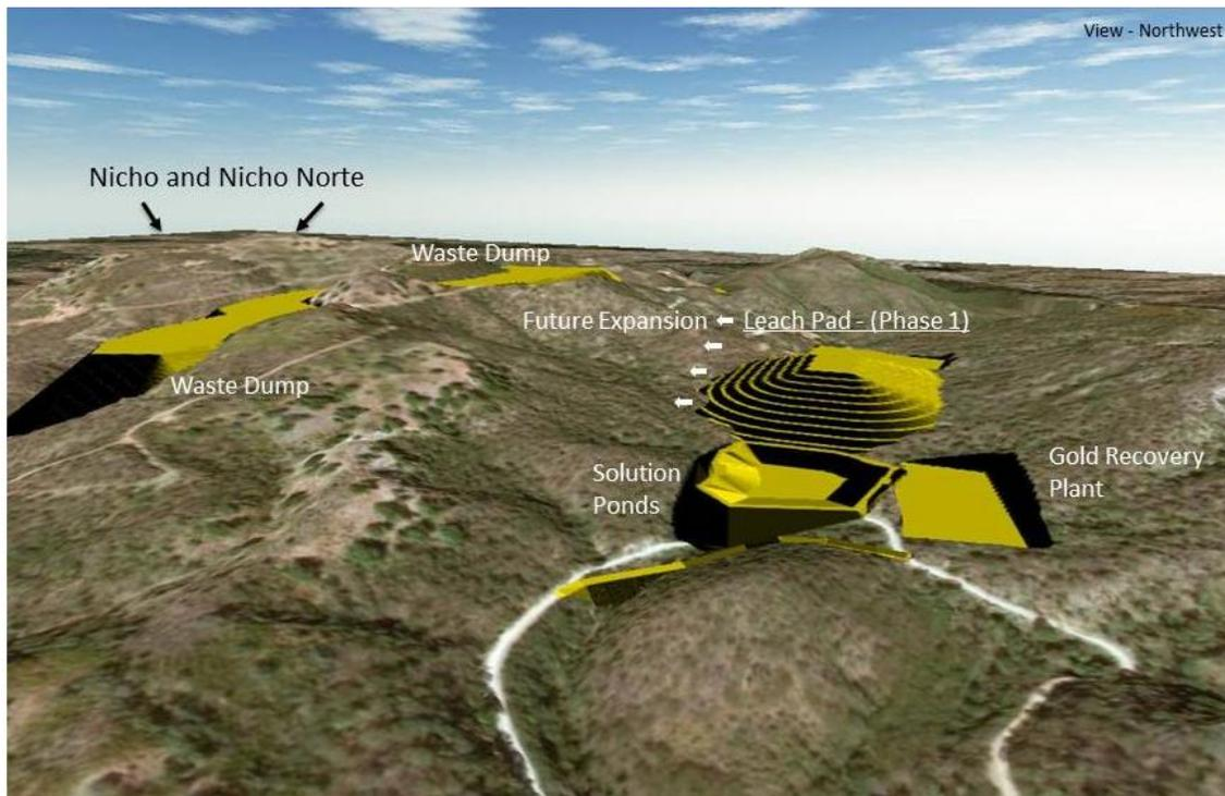
Figure 1 - Santana proposed gold heap leach operations site arrangement
