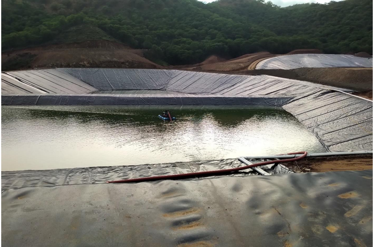
Photo 3 – The pregnant solution pond with floating pumping system in place and operational
